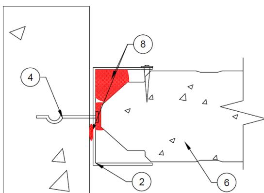
**Figure 32** - Male Panel End Detail for Vertical Speedpanel Wall
