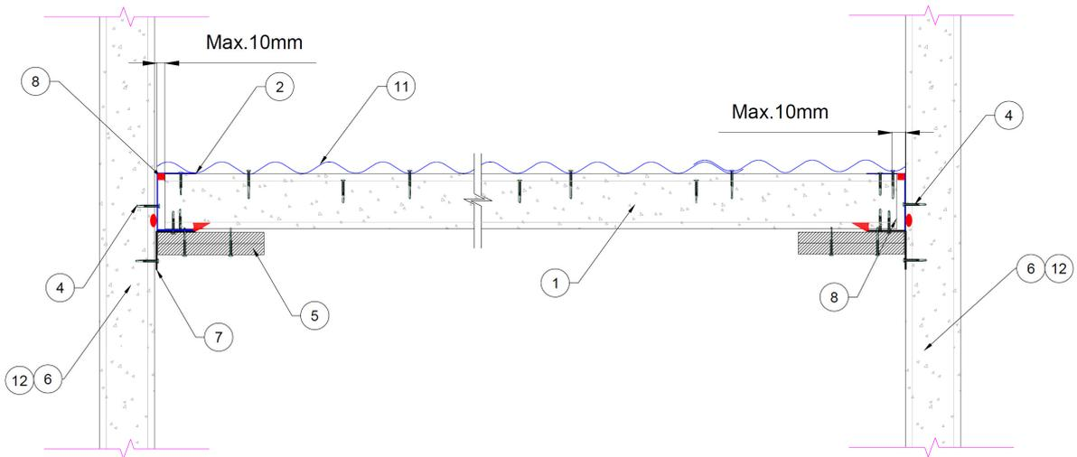
**Figure 11 –Speedpanel ceiling protected with steel sheeting (Longitudinal Section View)**
