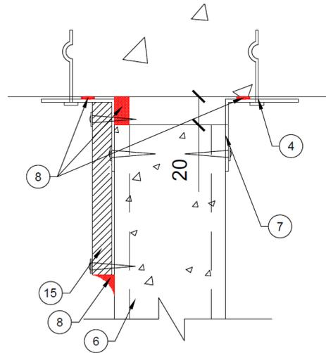
**Figure 29** – Head Detail for Vertical Speedpanel Wall
