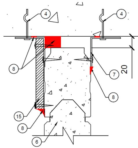
**Figure 39** – Head Detail for Horizontal Speedpanel Wall
