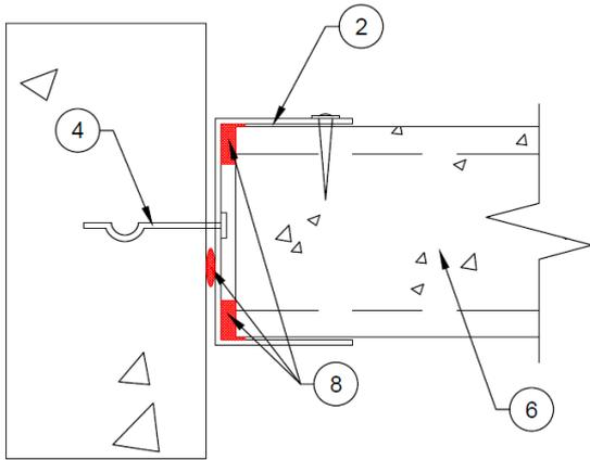
**Figure 34** – Cut-off Panel End Detail for Vertical Speedpanel Wall
