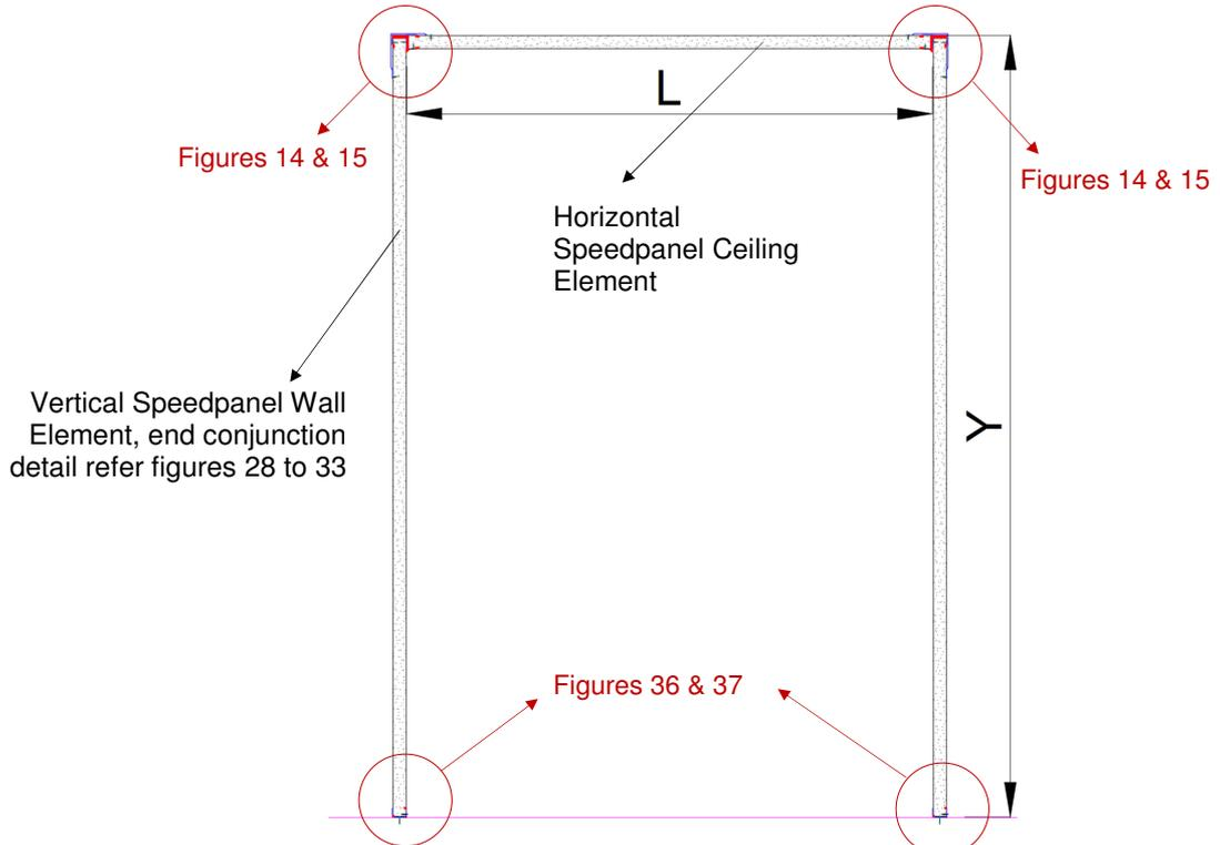
Figure 2 – Speedpanel ceiling and wall configuration
