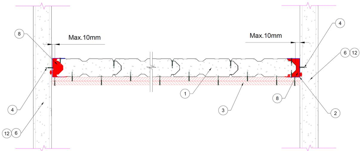
**Figure 12 –Speedpanel ceiling protected with plasterboard linings (Cross Section View)**
