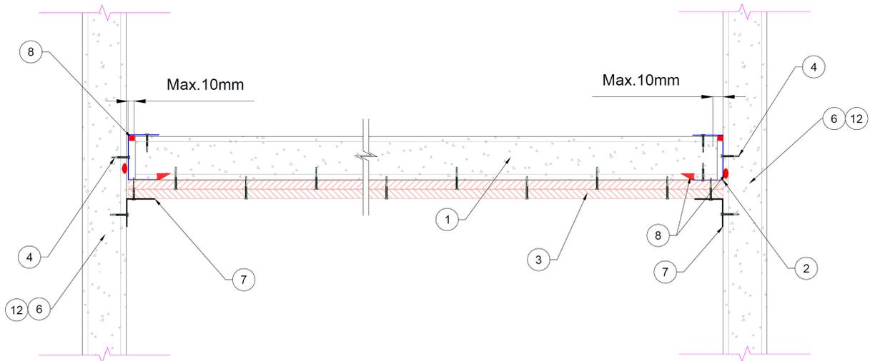
Figure 13 –Speedpanel ceiling protected with plasterboard lining (Longitudinal Section View)
