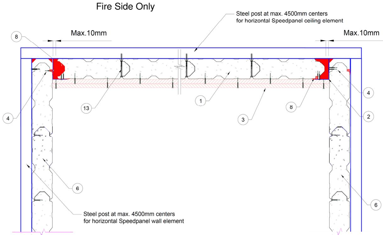
**Figure 22 –Speedpanel ceiling protected with plasterboard linings (Cross Section View)**
