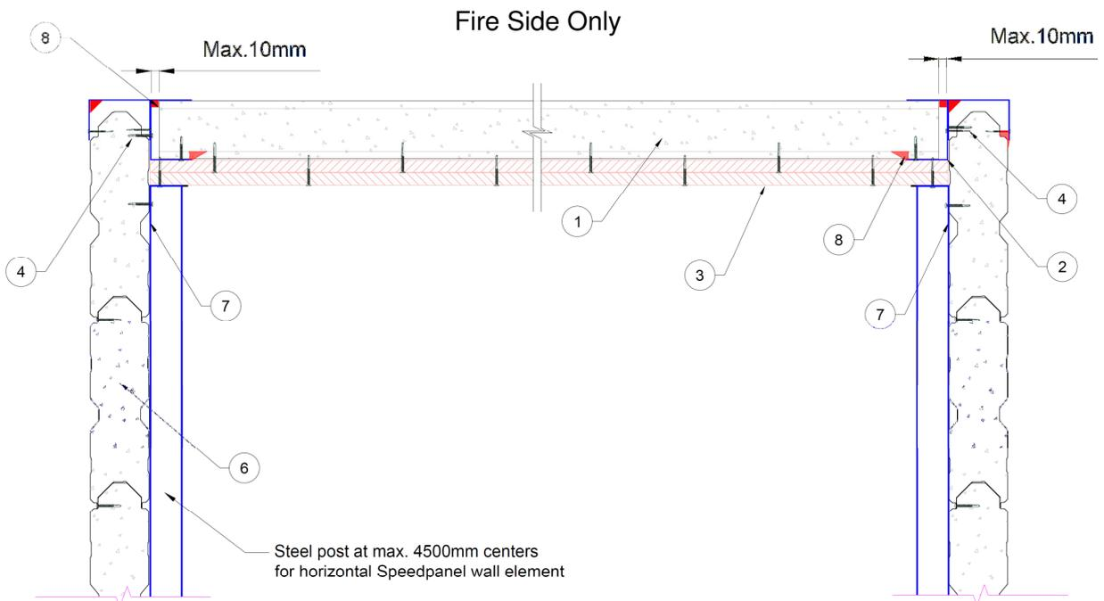
**Figure 23 –Speedpanel ceiling protected with plasterboard linings (Longitudinal Section View)**
