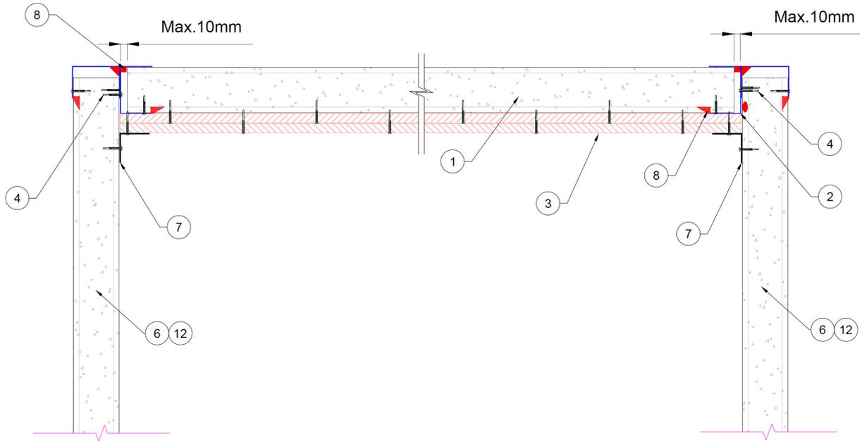
Figure 15 –Speedpanel ceiling protected with plasterboard lining (Longitudinal Section View)
