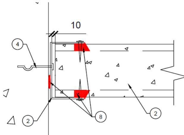
**Figure 40** – Side Detail for Horizontal Speedpanel Wall
