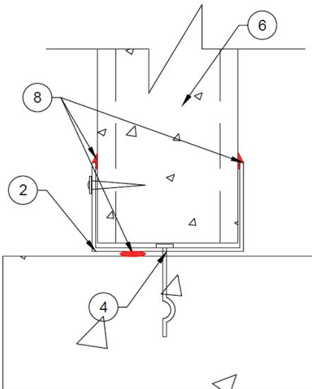
**Figure 36** – Bottom Detail for Vertical Speedpanel Wall
