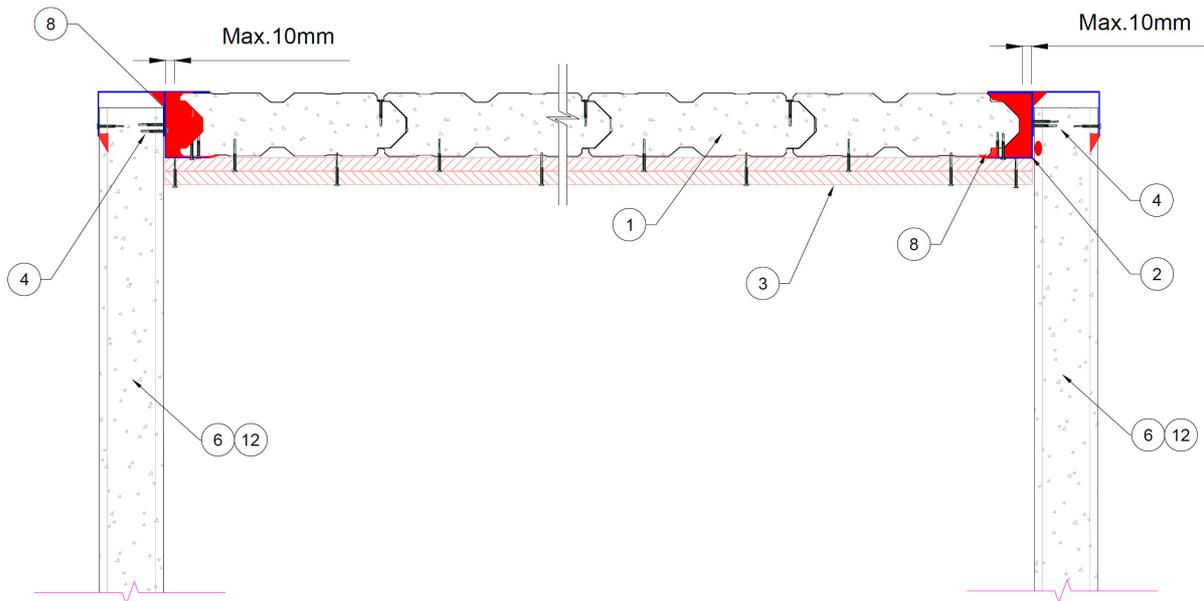
Figure 14 –Speedpanel ceiling protected with plasterboard linings (Cross Section View)
