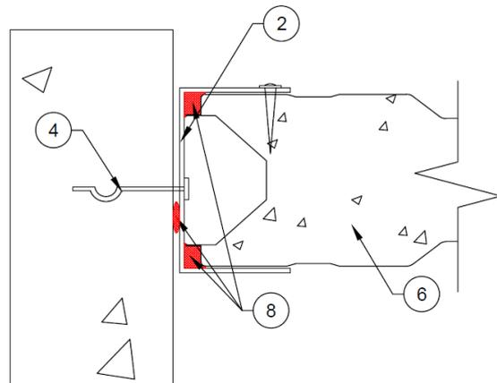
**Figure 31** - Female Panel End Detail for Vertical Speedpanel Wall
