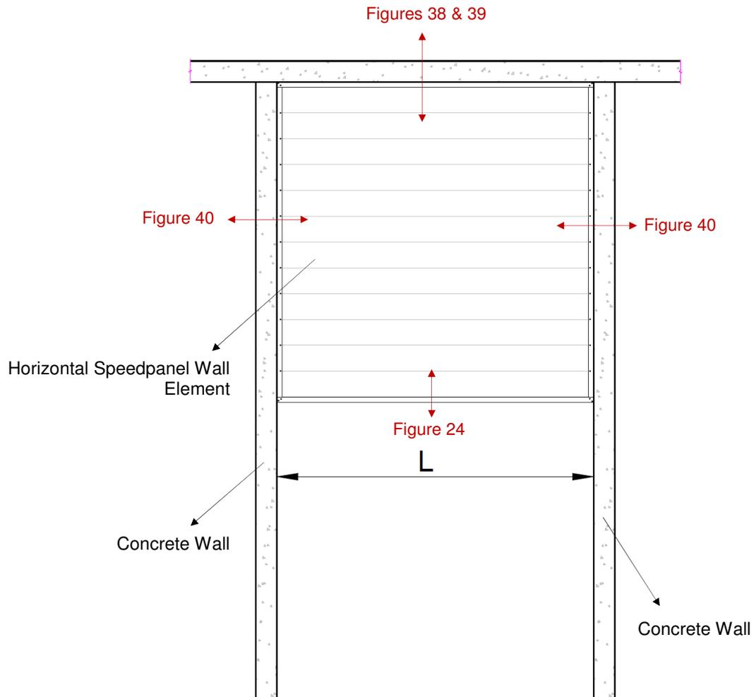
**Figure 7 – Speedpanel Bulkhead Configuration (Front View)**
