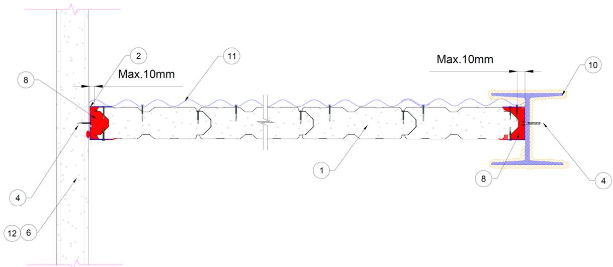
**Figure 18 –Speedpanel ceiling protected with plasterboard linings (Cross Section View)**
