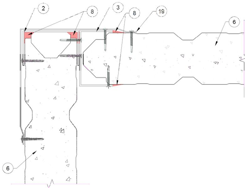
**Figure 45 – Corner Detail of Bulkhead Construction with two Vertical Speedpanel Walls**
