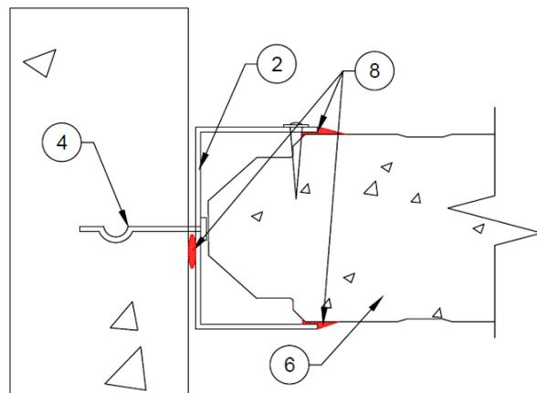
**Figure 33** - Male Panel End Detail for Vertical Speedpanel Wall
