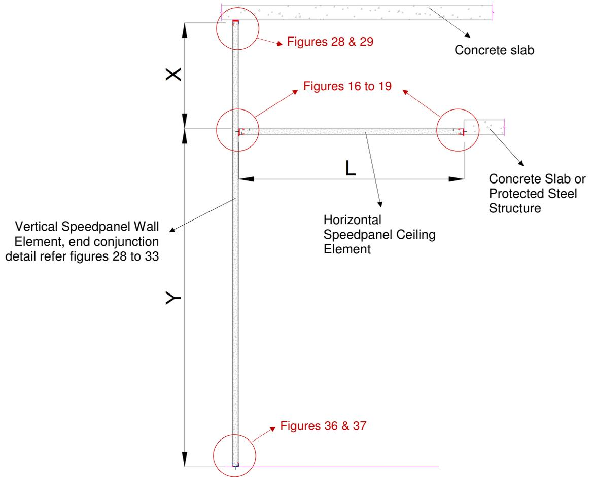
**Figure 3 – Speedpanel ceiling and wall configuration**
