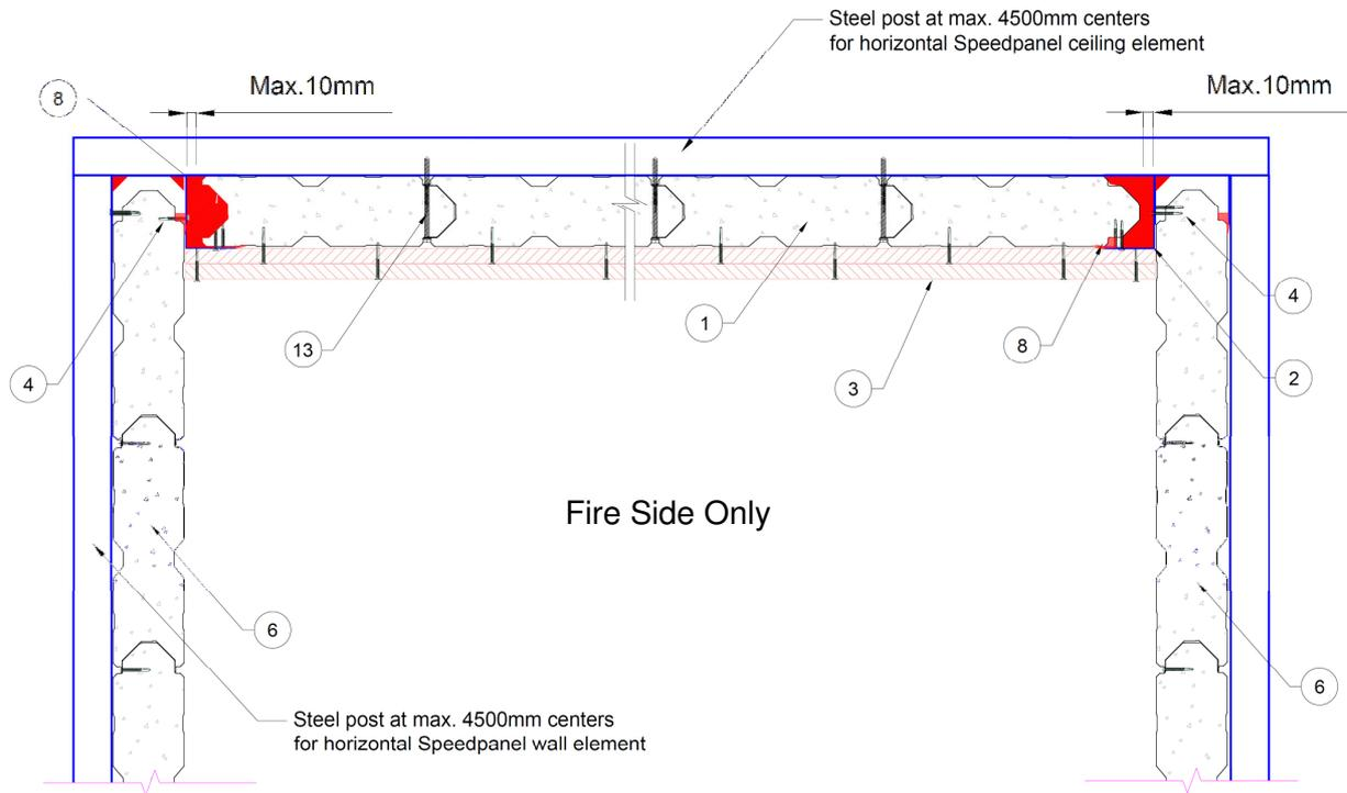
Figure 20 –Speedpanel ceiling protected with plasterboard linings (Cross Section View)
