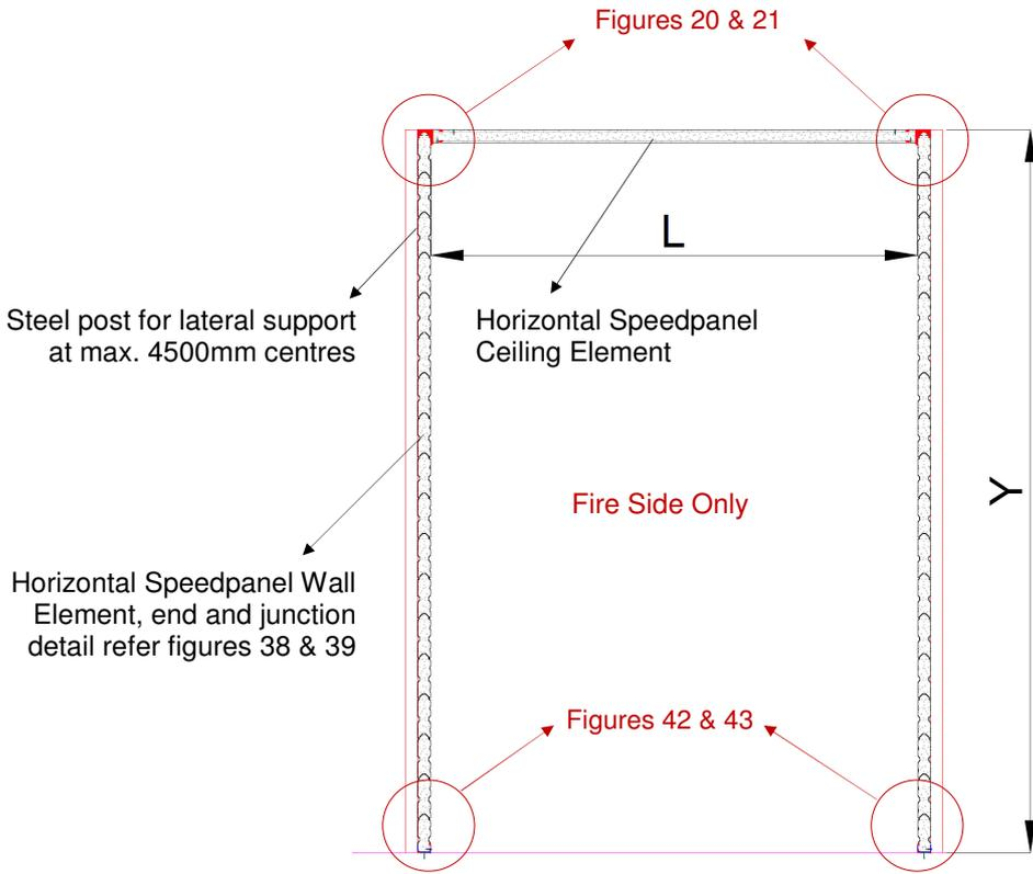
Figure 4 – Speedpanel ceiling and wall configuration
