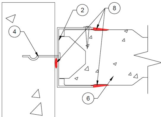
**Figure 30** - Female Panel End Detail for Vertical Speedpanel Wall
