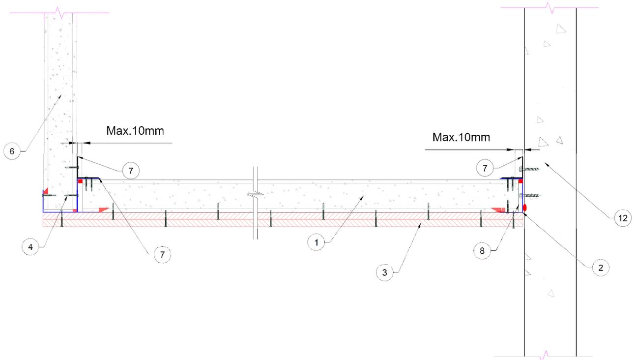
**Figure 27 –Speedpanel bulkhead ceiling span protected with plasterboard linings
