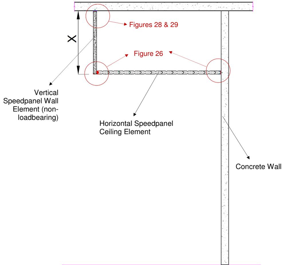
**Figure 8 – Speedpanel Bulkhead Configuration (Section Elevation View)**
