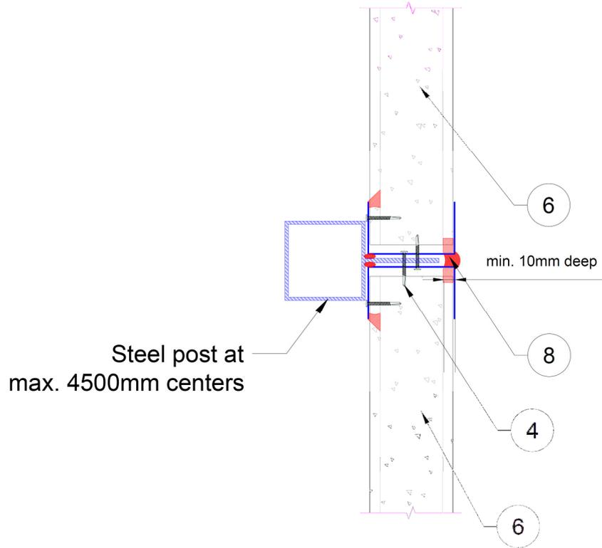
**Figure 41** – Junction Detail for Horizontal Speedpanel Wall and Steel Post
