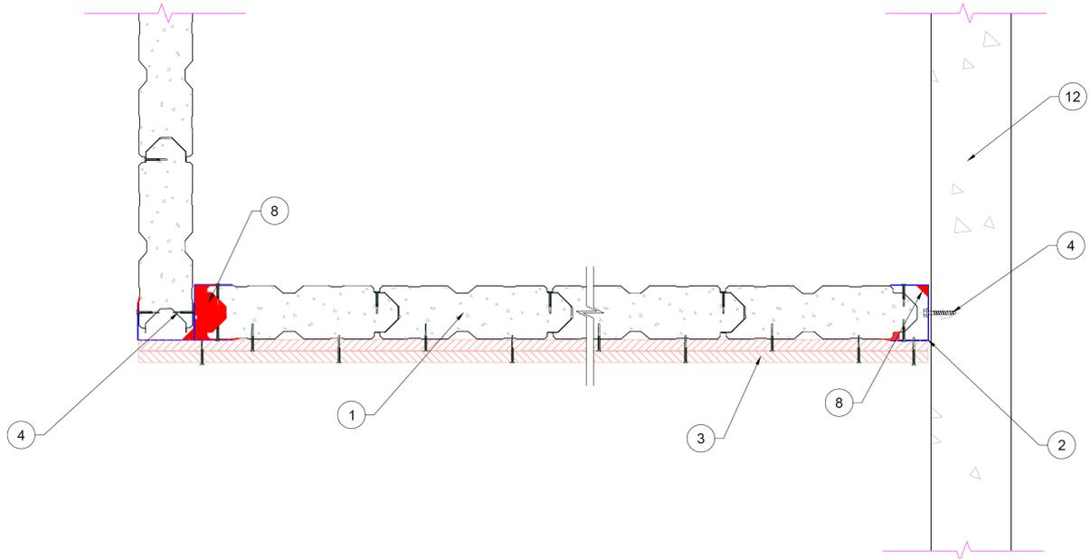
**Figure 24 –Speedpanel bulkhead ceiling span protected with plasterboard linings
