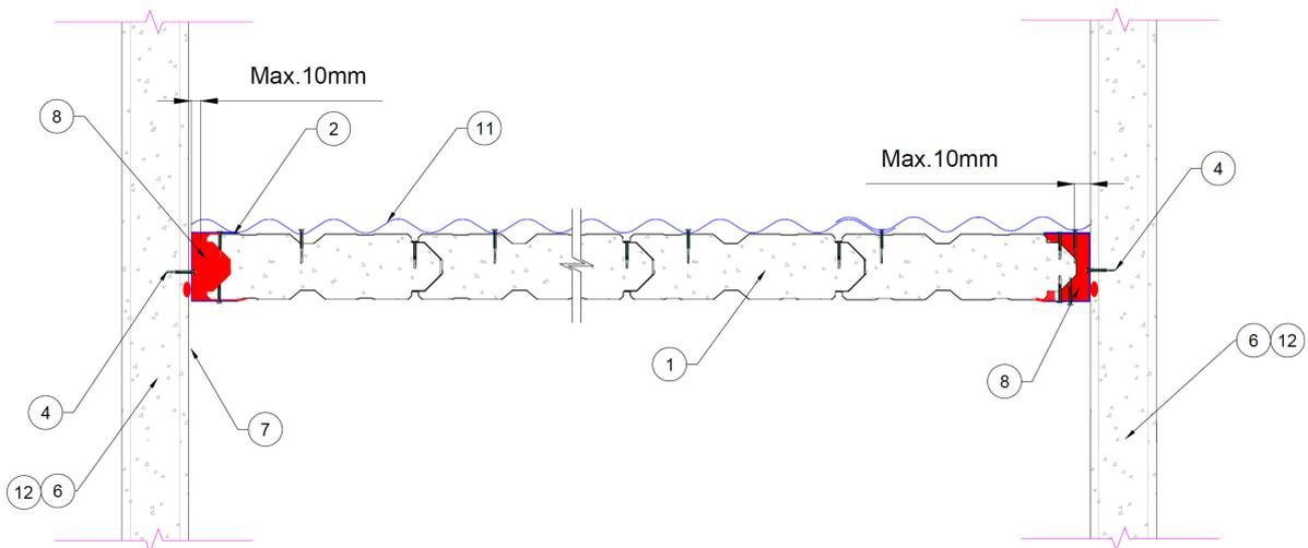
Figure 10 – Speedpanel ceiling protected with steel sheeting (Cross Section View)
