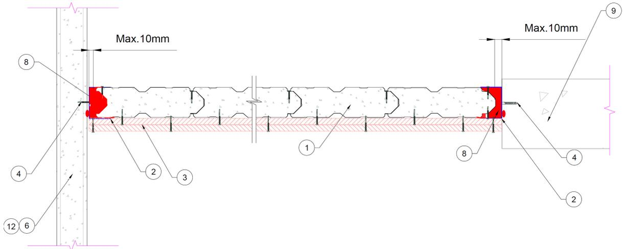
Figure 16 –Speedpanel ceiling protected with plasterboard linings (Cross Section View)
