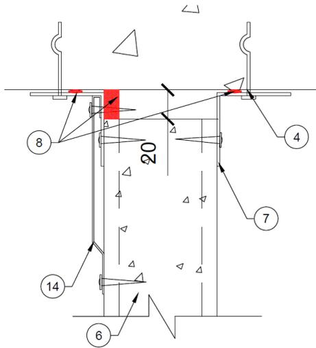
**Figure 28** –Head Detail for Vertical Speedpanel Wall
