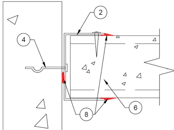
**Figure 35** – Cut-off Panel End Detail for Vertical Speedpanel Wall
