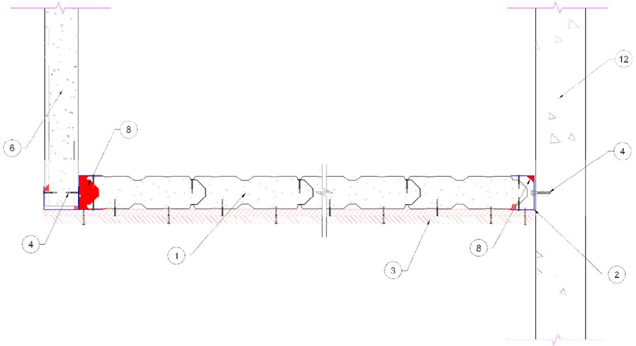
**Figure 26 –Speedpanel bulkhead ceiling span protected with plasterboard linings
