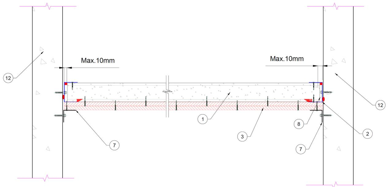
**Figure 25 –Speedpanel bulkhead ceiling span protected with plasterboard linings
