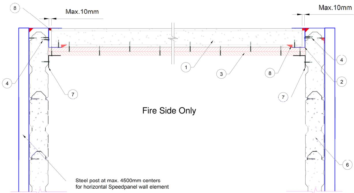
Figure 21 –Speedpanel ceiling protected with plasterboard linings (Longitudinal Section View)
