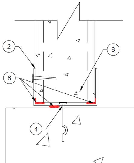
**Figure 37** – Bottom Detail for Vertical Speedpanel Wall
