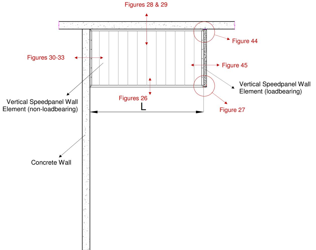
Figure 9 – Speedpanel Bulkhead Configuration (Front View)
