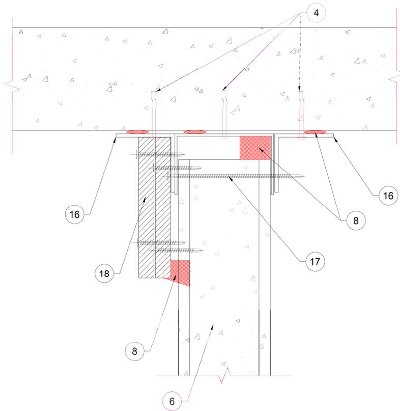
**Figure 44 – Head Detail for Suspended Vertical Speedpanel Wall**
