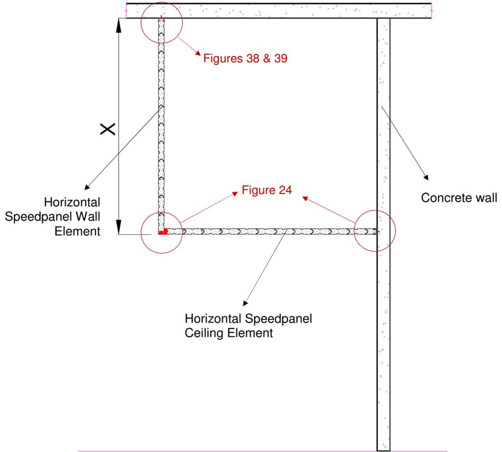
**Figure 6 – Speedpanel Bulkhead Configuration (Section Elevation View)**
