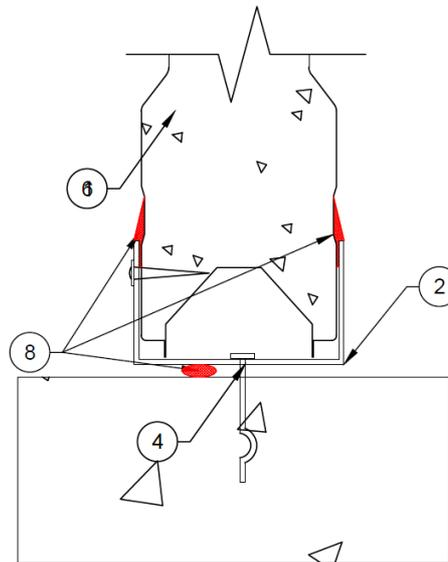
**Figure 43** – Bottom Detail for Horizontal Speedpanel Wall
