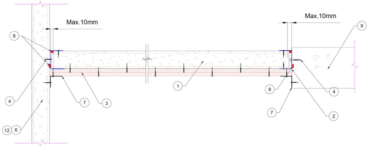
**Figure 17 –Speedpanel ceiling protected with plasterboard linings (Longitudinal Section View)**
