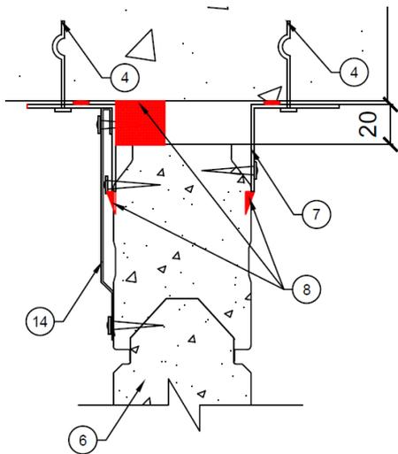
**Figure 38** – Head Detail for Horizontal Speedpanel Wall
