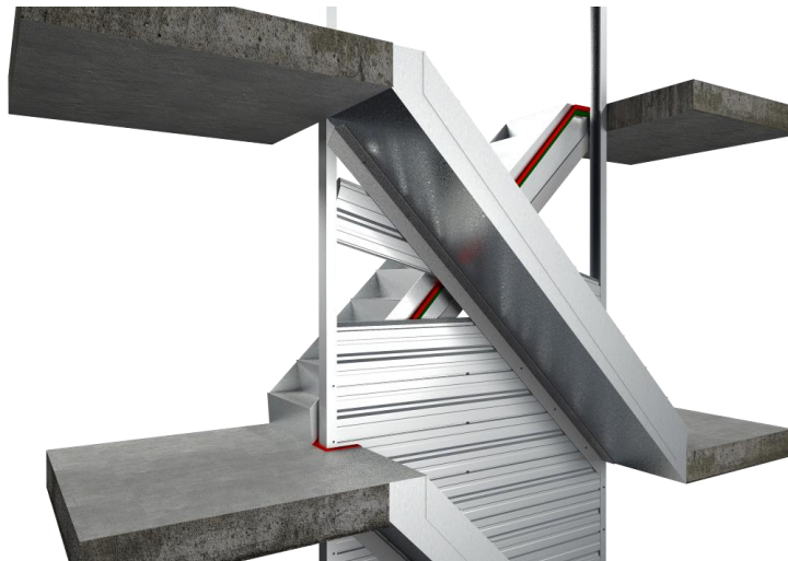
Figure 2: Scissor stair configuration during assembly, steel angle at bottom
