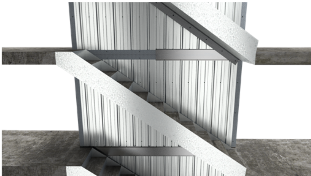
Figure 8 Single 78 mm thick vertically stacked wall – steel angle at bottom of stringer
