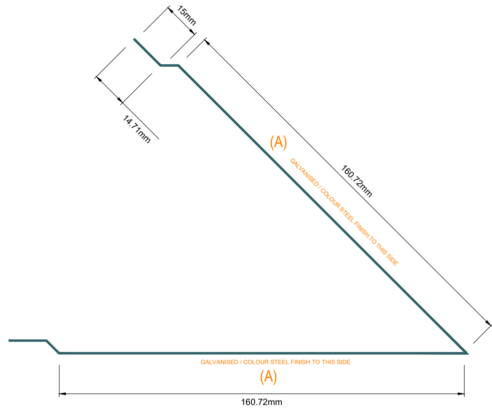
SPEEDPANEL® External Corner Flashing Acute 1.15mm BMT
